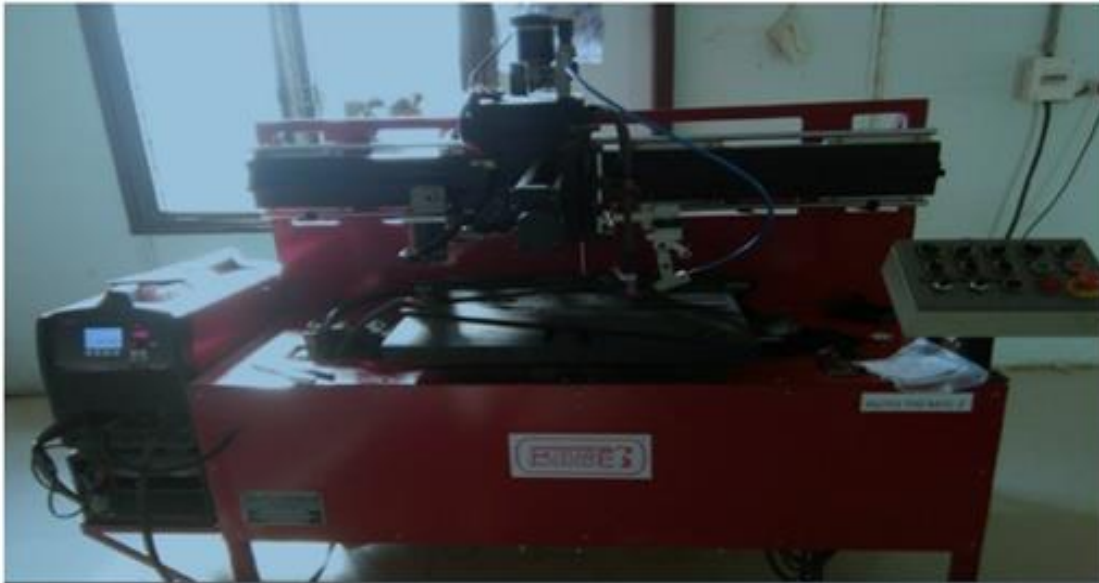
Figure 1: Automatic TIG welding Machine
