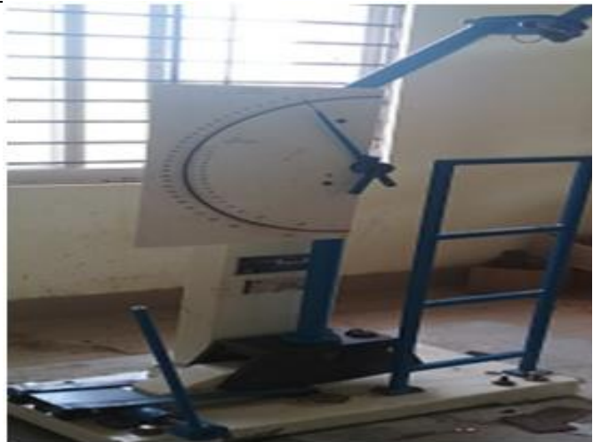
Figure 3: Impact test to measure toughness
